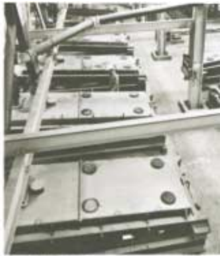
Bank of 17 ROTEX Screeners sizing potash at Potash Division, Cominco, Ltd. Saskatchewan, Canada
