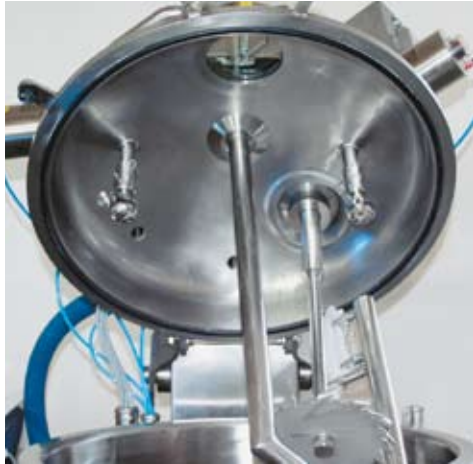
Agitator with vortex breaker
