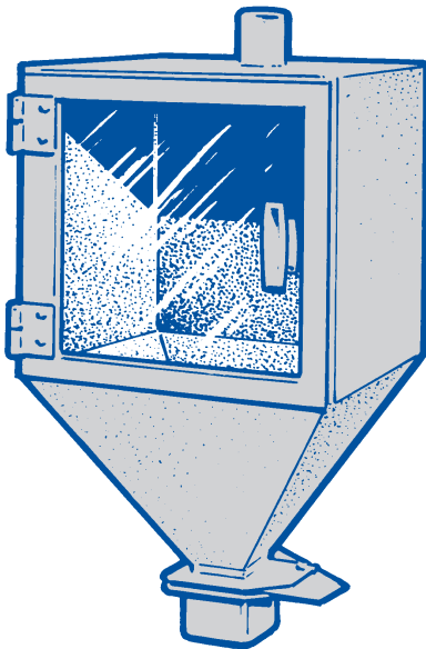
HOPPER STYLE — INCLUDES HINGED PLEXIGLAS DOOR AND A SLIDING MANUAL GATE.
